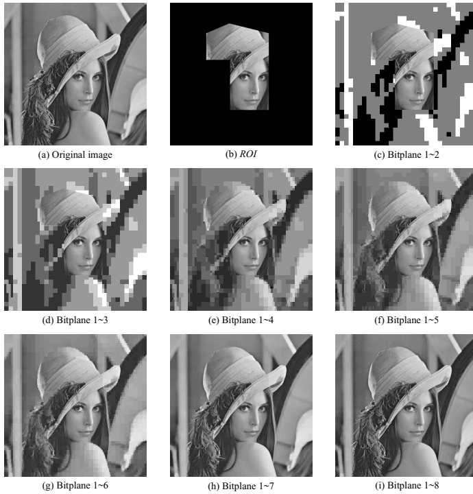
Fig. 5. Progressive lossy-to-lossless coding with polygon-shaped ROI
