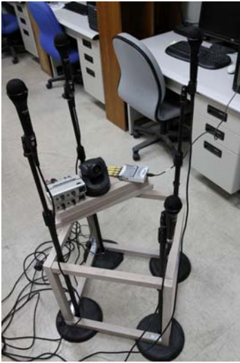
Fig. 3. The 4-microphone tracking system
