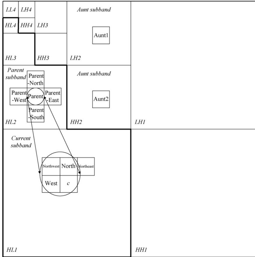
Fig. 2. The relation map for computing correlation between coefficient  $c$  and the coefficients in the parent, aunt, and current subbands.
