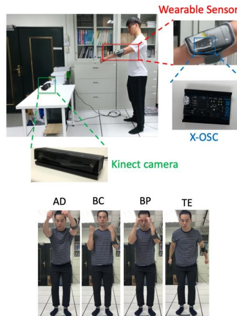
Fig. 2. The environment of the mounted camera and the worn sensor device; the fitness behaviors: anterior deltoid (AD), biceps curl (BC), back pullover (BP), and triceps extension (TE).
